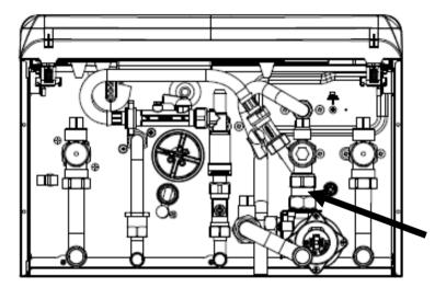
Boiler Adaptor (6) to be used on InTec 30/34C models.
