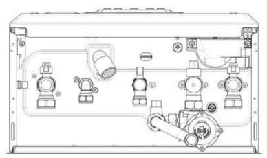
Cyclone assembly fitted to an E-Tec/Evoke & ECO<sup>2</sup>
